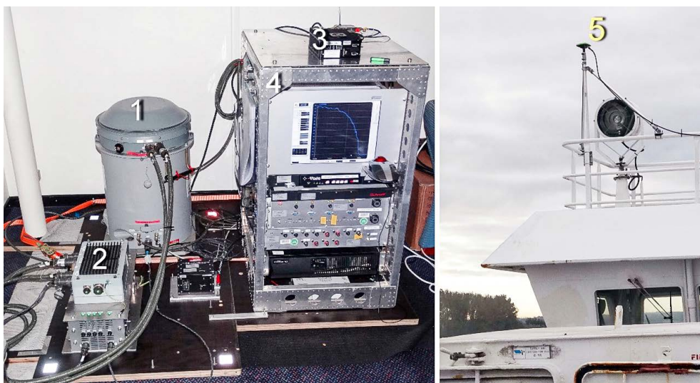
Fig. 1: Installation of GFZ's Chekan-AM gravimeter onboard the ferry Stena Line Urd. The main components are the Chekan sensor (1), power supply (2), Javad GNSS receiver (3), a rack (4) with various control computers and an uninterrupted power supply and one of the Javad GNSS antennae on top of the wheelhouse (5).
