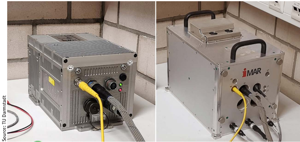
Fig. 2: The iNAV-RQH-1003 strapdown gravimeter of TU Darmstadt (left) and the thermal stabilization housing iTempStab-AddOn used for this strapdown instrument (right).
