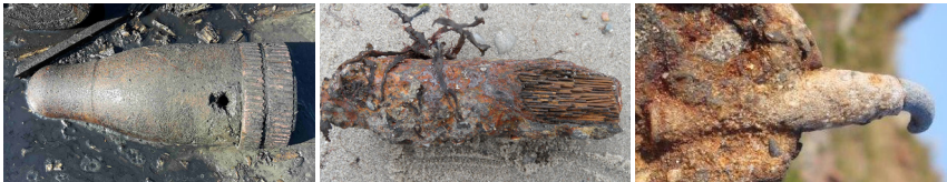
Fig. 2: From North and Baltic Sea (left to right): grenade, burst, 2016 – rusted British cartridge case, 2015 – grenade, embedded in concrete, 2013
