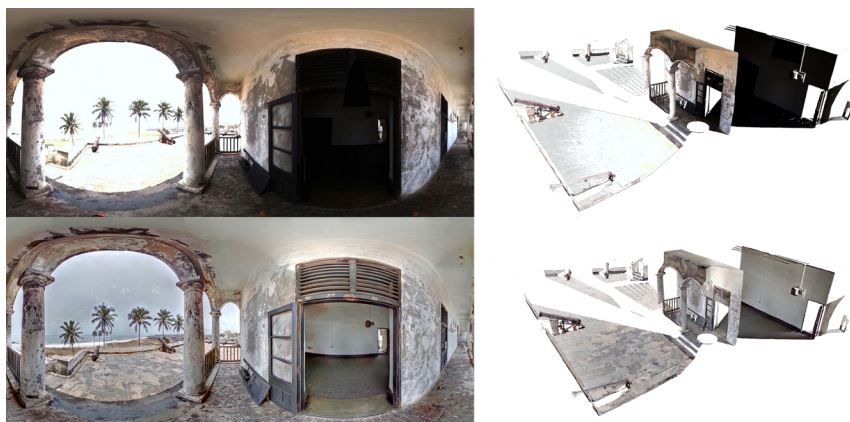
Fig. 3: Panoramic image taken with a Z+F IMAGER 5010C (left) and the according 3D scan (right), taken without HDR (above), with HDR (below) at Elmina Castle, Ghana, Zamani Project
