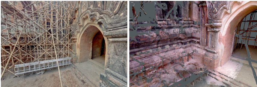
Fig. 9: Left: Colour image of the bamboo scaffolding taken with the Z+F scanner. Right: Filled-in data with the DPI-8-handheld scanner
