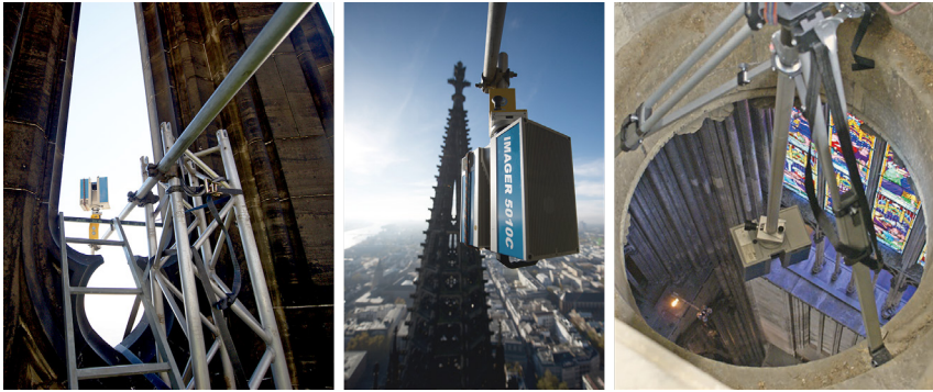
Fig. 6: Moveable extension rig at North tower, Cologne cathedral, to scan tower tips above (left) and below (centre). Inverted setup over keystone opening (right)
